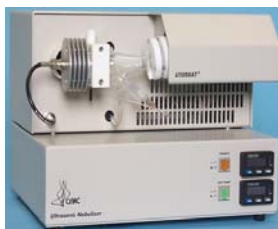
Figure 4 - CETAC U-5000AT+ Ultrasonic Nebulizer
